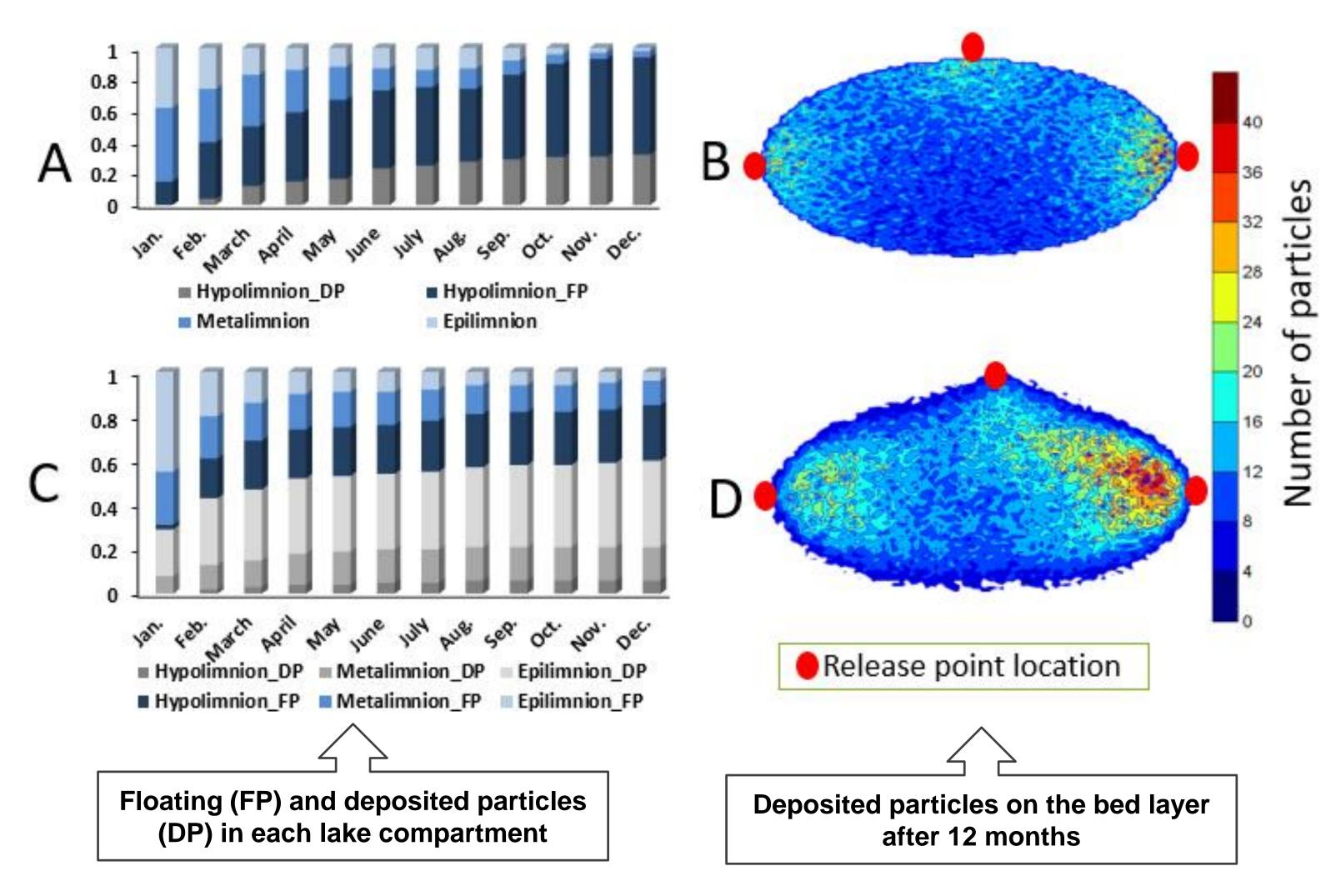
The simulation results are depicting the deposited MPs and Floating MPs for the constant (A&B) and oval-shaped (C&D) bathymetries, respectively.
